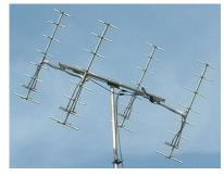
of packing and transportation. The Quad Yagi Array is supplied with complete mounting hardware balanced at its center of gravity for mounting on a rotator for azimuth and elevation plane scanning. The mounting hardware supplied is of stainless steel fasteners and three aluminum cross members for stacking.
